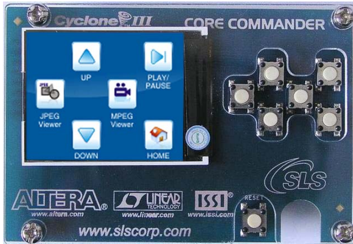
Figure 15 : Picview Application Running on CoreCommander Board
