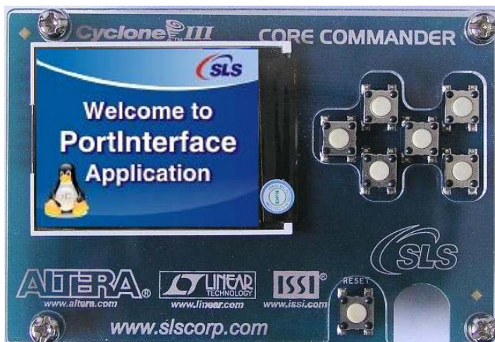
Figure 25 : CoreCommander board Startup Screen Running PortInterface Appl.
