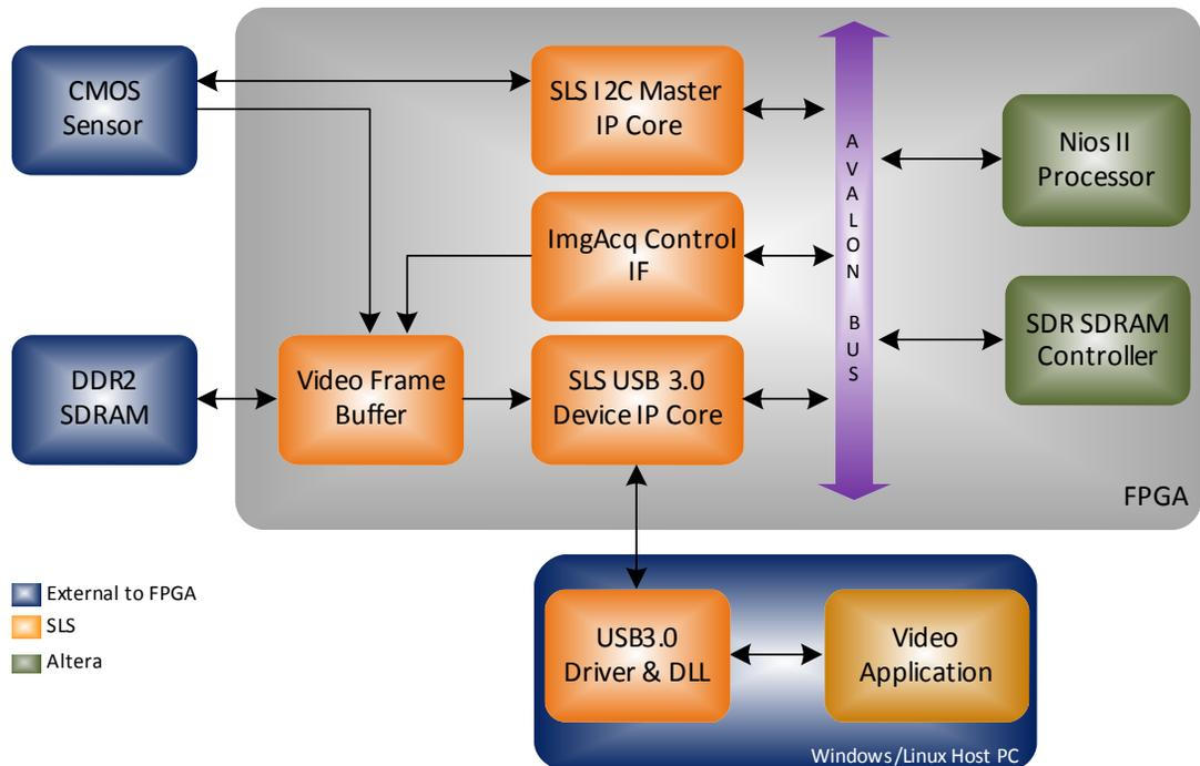
As shown in the block diagram, a CMOS camera sensor data is being transferred over USB 3.0 interface using SLS USB 3.0 Device. The Nios II processor is used to control peripherals such as memory controller, I2C master and enumeration of the USB 3.0 Device on Host PC running with Windows or Linux Operating System (OS).
