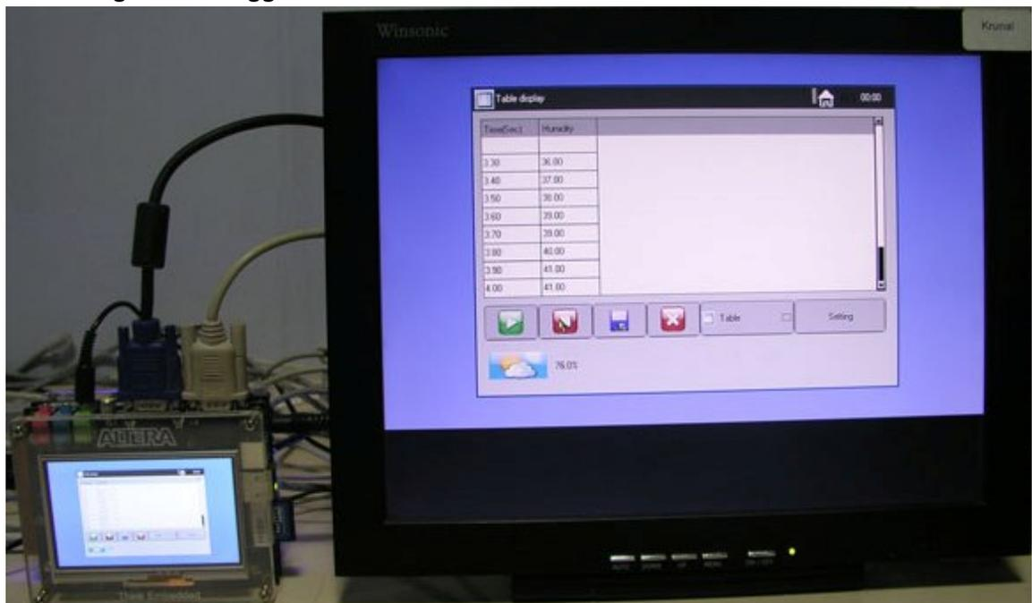
8. To change sampling frequency click on Settings button. Enter the desired frequency. See [Figure 29](#) below.
